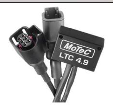
MoTeC's LTC (Lambda To CAN) monitors, controls and diagnoses a Bosch LSU 4.9 Lambda sensor, and transmits Lambda readings on a CAN bus. When using LTCs, up to 32 Lambda sensors can be configured on a single CAN bus allowing an ECU or logging device to simultaneously monitor multiple Lambda sensors.
