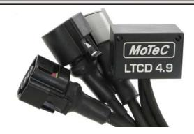
MoTeC's LTCD (Lambda To CAN) is the twin version of the LTC (#61300). It monitors, controls and diagnoses two Bosch LSU 4.9 Lambda sensors, and transmits Lambda readings on a CAN bus. When using dual LTCs or a mix of singular and dual LTCs, up to 32 Lambda sensors can be configured on a single CAN bus to simultaneously monitor multiple Lambda sensors.
