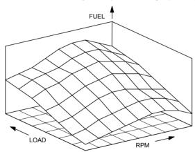
The ECU determines the amount of fuel to inject by first calculating the RPM and Load then extracting the corresponding value from the table. If the RPM and Load do not match an RPM and LOAD point exactly then the values from the closest sites are mathematically interpolated to arrive at an intermediate value.
