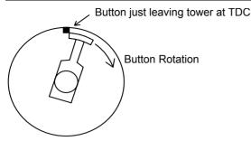
The button must be a wide tip type to cater for a wide range of advance points since the advance is changed electronically rather than mechanically.
