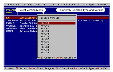
To check which version of the software a particular ECU is running, start the latest version of the E.M.P. Software. If the ECU is not the correct type or the ECU software version does not match, then a screen will be displayed that will show the current ECU type and version.
