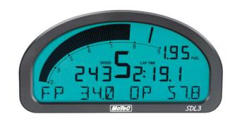
The Sport Dash Logger (SDL3) comes standard as a combined display and powerful control device in one lightweight unit. With the addition of the Data Logging upgrade it becomes a fully programmable data logger with a 16 or 120 MB memory.
