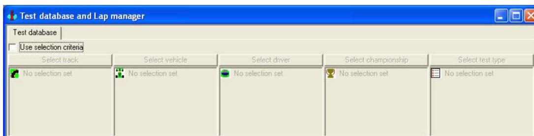
Fig. 3.4– *Test database and Lap manager* window: "selection criteria" option disabled
