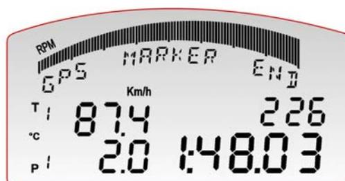
Starting from this moment **MyChron3 Dash** automatically samples lap/split times using the GPS signal only.
