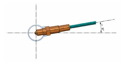
Once the probe is installed, pay attention not to let the cable pass near to excessive heat sources (the exhaust pipe for example).
